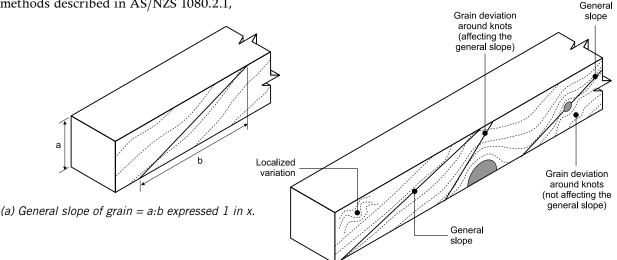
Figure C.2 Measurement of slope of grain
