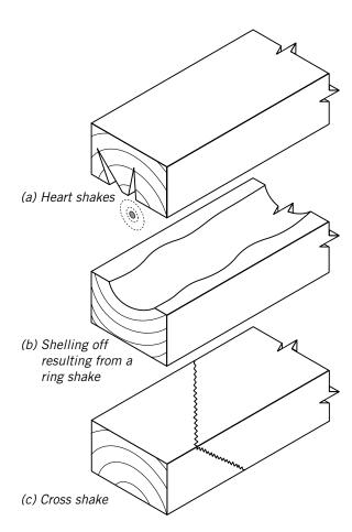
Figure C.4 Checks and splits Figure C.5 Shakes
