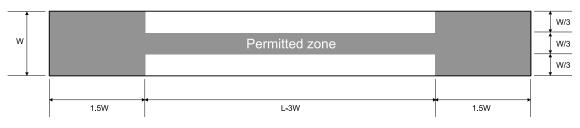
Figure 3.5 Permitted zones for notches in beams
