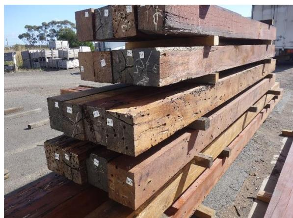
Heart is the dead centre of a sawlog often defined by a star fracture. It is the pith, corewood or growth heart of a living tree and is responsible for significant internal tension as the sawlog dries. It should not be confused with heartwood or truewood – which is the good stuff we all like.
